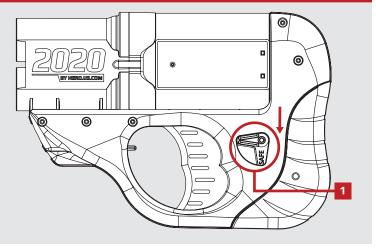
Before your device can be fired the safety switch must be disabled. You can access the safety from either side of the device.
